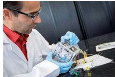
Propellant management assembly Copyright : Air Liquide – Laurent Lelong
